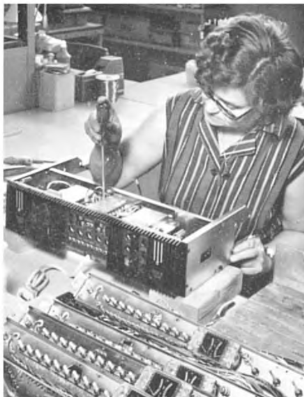
Fig. 2. Assembly of the T9000 integrated tuner amplifier. From this illustration it can be seen that the device is built as a single unit, although the final styling emphasises the separateness of the tuner and amplifier sections
